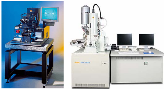
Figure 3.3: SUSS MJB4 Manual Mask Aligner for micron size resolution and HR-SEM Jeol JSM 7000F for sub micron patterning resolution.
