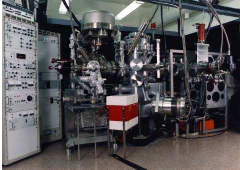
Figure 3.1: The electron beam coevaporation system for sample growth.
